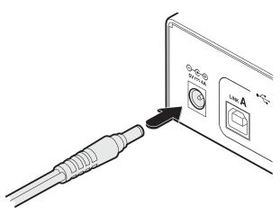
Note: Both the unit and its power supply generate heat when in operation and will become warm to the touch. Do not enclose them or place them in locations where air cannot circulate to cool the equipment. Do not operate the equipment in ambient temperatures exceeding 40 degrees Centigrade. Do not place the products in contact with equipment whose surface temperature exceeds 40 degrees Centigrade.
