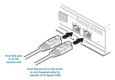
2 If Hi-Speed USB is required, connect the CATx link cable from port B of the receiver unit to port B on the front panel of the transmitter unit.
