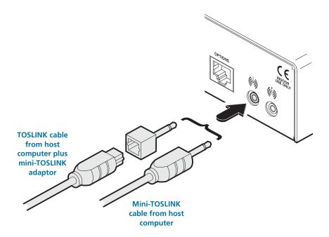
Note: This digital input is fed across the main CATx link to the optical connection of the receiver's Line Out socket only. There is no crossover between the analog and digital audio subsystems of the Wizard DP Extender installation.
