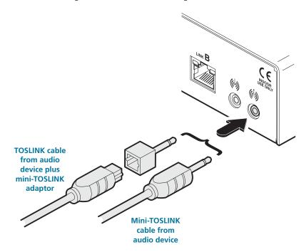
Note: This digital output is fed via the main CATx link from the optical connection of the transmitter's Line In socket only. There is no crossover between the analog and digital audio subsystems of the Wizard DP Extender installation.
