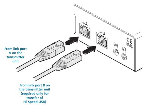
2 If Hi-Speed USB is required, connect the CATx link cable from port B (on the front panel) of the transmitter unit to the LINK B port on the rear panel of the receiver unit.
