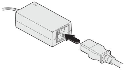
3 Connect the power lead to a nearby mains supply socket.
