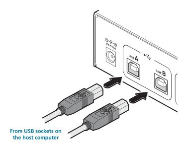
2 If the USB port B is required (on the receiver unit), use the second supplied USB cable to connect the Link B socket on the rear panel of the transmitter unit with a vacant USB socket (v2.0) on the host computer.
