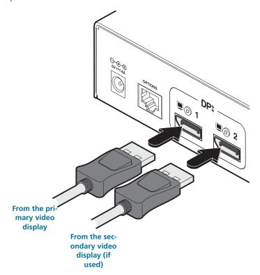
2 If a second video display is to be used, connect its cable to the DP++ port 2 on the rear panel of the transmitter unit. If an adaptor is required, see above.
