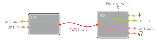
You can choose between these two analog inputs using a hotkey switch, as follows:
