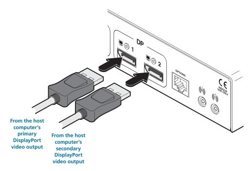
2 If a second video display is required, use an additional DisplayPort video cable to link DP port 2 on the rear panel of the transmitter unit with the secondary video output socket of the host computer.
