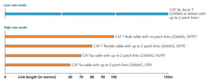
As mentioned above, patch links affect performance. For each additional break/patch within a run, you will need to reduce the distance given above by roughly 5 meters.
