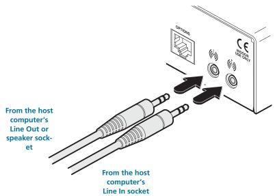
2 If a microphone or other audio input is required (from the Wizard DP Extender receiver back to the host computer), use another 3.5mm jack audio cable to connect the Line Out (i) socket on the transmitter to the analog Line In socket of the host computer
