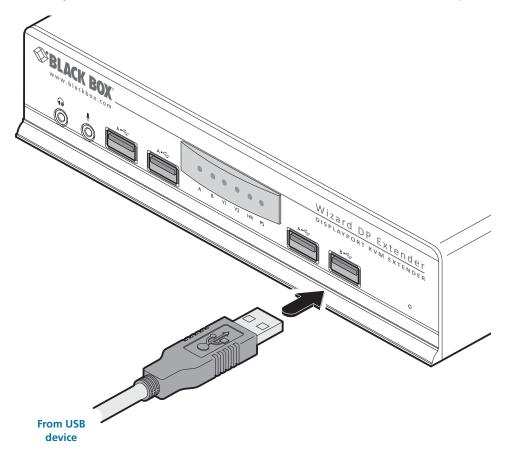
For Hi-Speed USB peripherals, such as mass storage devices, use socket B 😋
