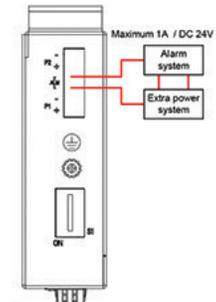
Figure 3-4. Alarm relay output contacts on the LIG401A.
