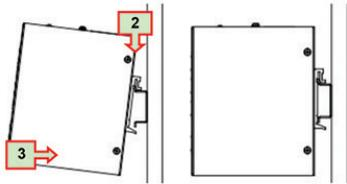
Figure 3-1. Din-rail mounting.
