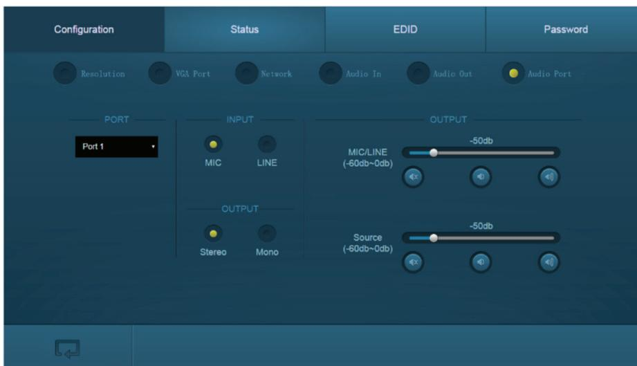
FIGURE 6-14. CONFIGURE PGM OUT AUDIO PORT
