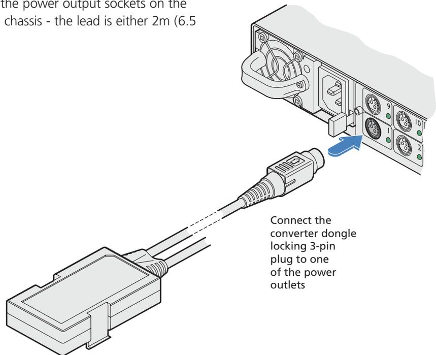
Connect the converter dongle locking 3-pin plug to one of the power outlets
