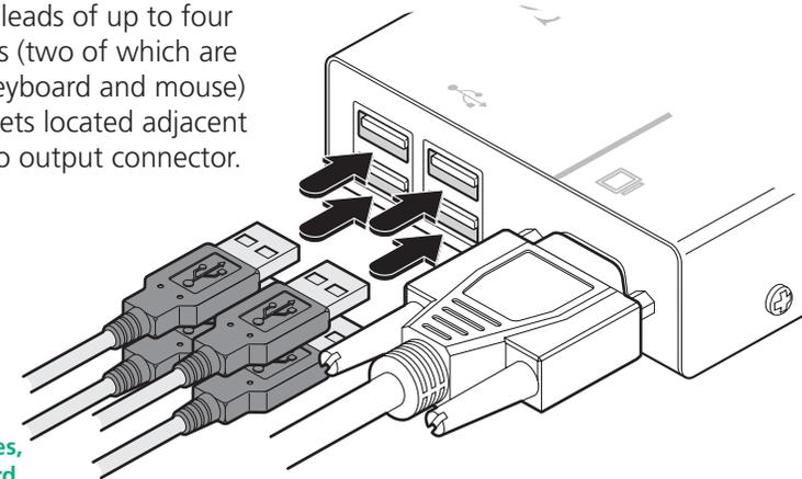
[MS2 variant only] Note: When connecting four USB devices to the unit, ensure that their total power requirements do not exceed 1700mA (1.7A). The USB standard states a maximum allowable current draw of 500mA (0.5A) per device, although most devices remain well below this limit - USB keyboards and mice typically require 100mA. Each X50 contains a self-resetting fuse that will prevent damage by shutting down the unit if the total power draw becomes excessive.
