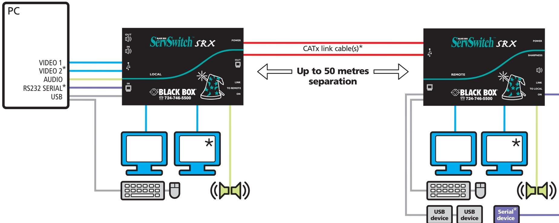
\* Secondary video, RS232 serial and a second link cable are available only with the Wizard SRX Dual VGA variant
