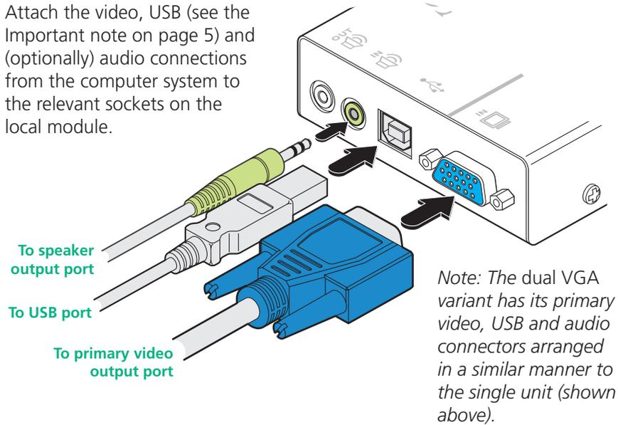
Note: Do not use a USB cable that is longer than 3 metres to connect the local module to the computer system.
