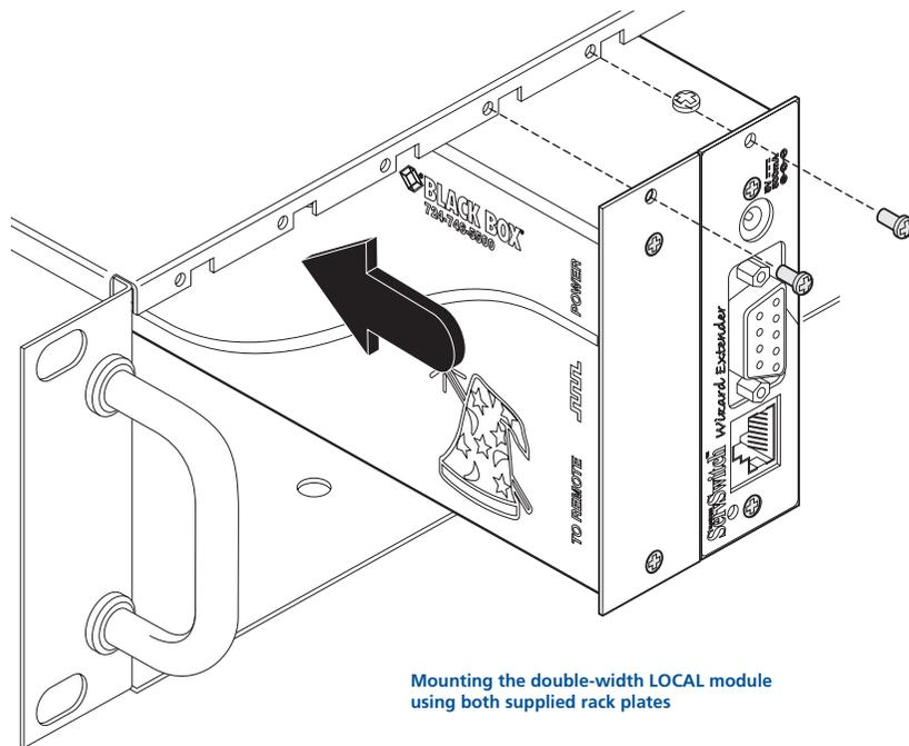
Mounting the double-width LOCAL module using both supplied rack plates
