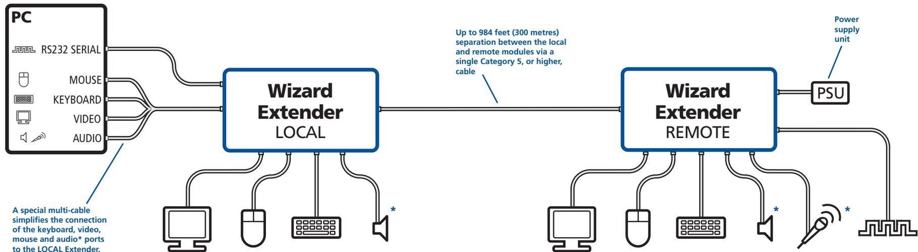
A special multi-cable simplifies the connection of the keyboard, video, mouse and audio\* ports to the LOCAL Extender.
