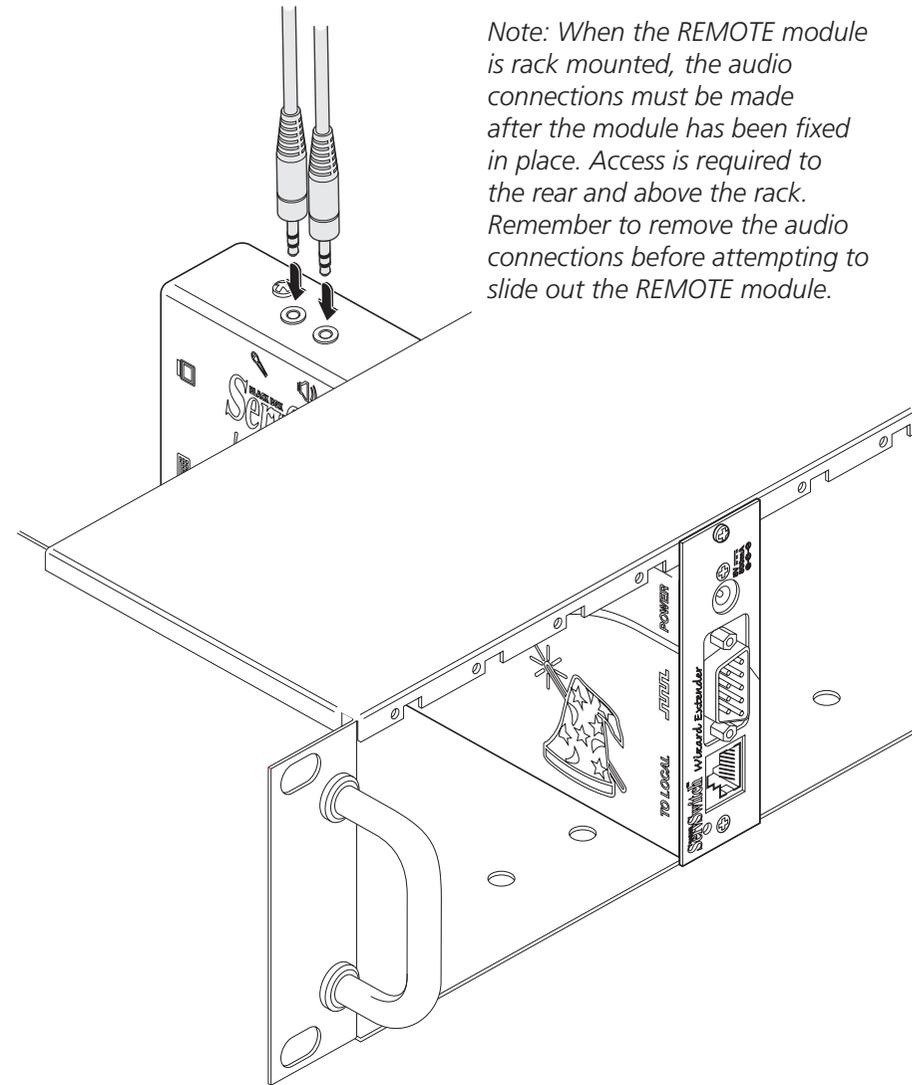
Note: When the REMOTE module is rack mounted, the audio connections must be made after the module has been fixed in place. Access is required to the rear and above the rack. Remember to remove the audio connections before attempting to slide out the REMOTE module.
