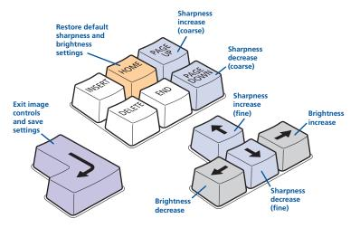
4 When no shadows are visible and the displayed images have crisp edges, press to exit configuration mode and permanently save all settings.
