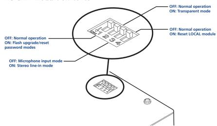
Note: When shipped, all switches are set in the OFF positions and this will produce normal operation with normal microphone input (at the REMOTE module).
