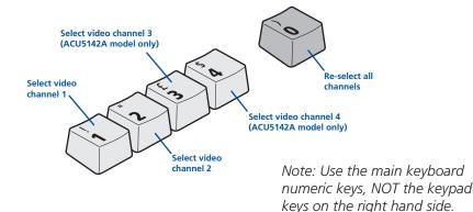
Note: When entering configuration mode, all video channels are automatically selected. You can change the video channel at any time.
