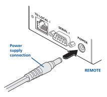
2 Insert the IEC connector of the supplied power lead into the corresponding socket of the power supply. Connect the other end of the power lead to a nearby mains socket.
